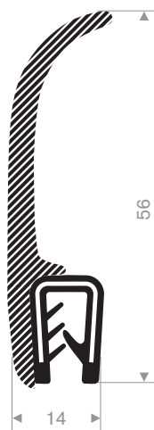
245.00.876 pvc + mosrubber klembereik 1-3 mm
