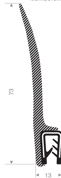
245.00.877 pvc + mosrubber klembereik 1-2 mm
